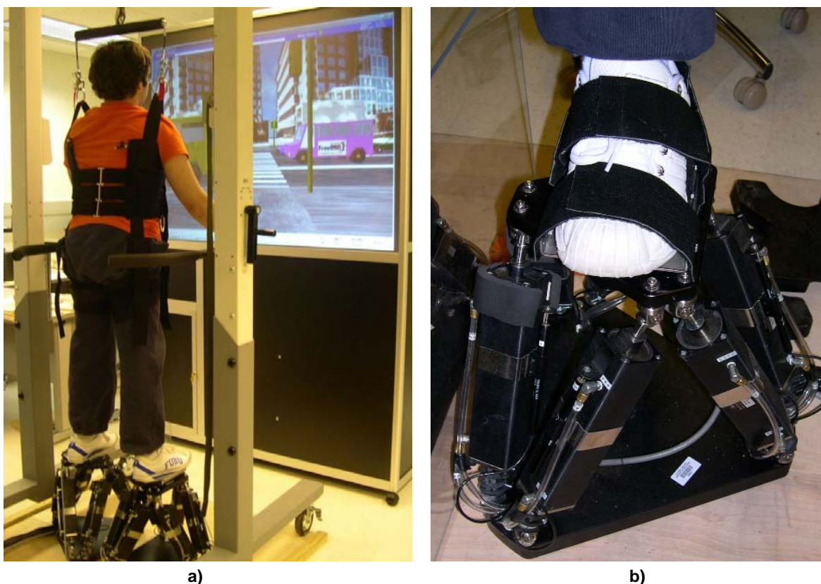
Figure 1. The -VE Mobility Simulator: a) general view; b) Rutgers Mega-Ankle (RMA) haptic device. © 2004 Rutgers University and UMDNJ. Reprinted by permission.
