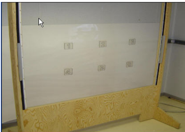
Figure 3 Physical target grid for virtual environment calibration.
